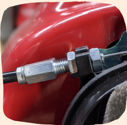
Figure 6: Jam nuts in the "forward" position
