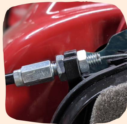
Figure 7: Jam nuts in the "backwards" position
